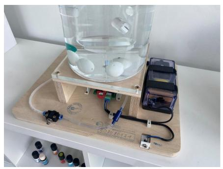
Loosen all wires/hoses that go to the pump. The power supply of the pump comes from the lamp. You can pull the green crown stone loose so that you can easily unscrew the cable of the pump.
