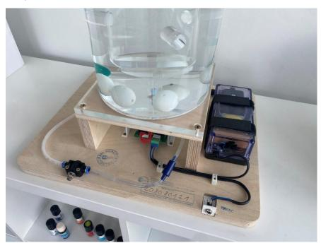
Loosen all wires/hoses that go to the pump. The power supply of the pump comes from the lamp. You can pull the green crown stone loose so that you can easily unscrew the cable of the pump.
