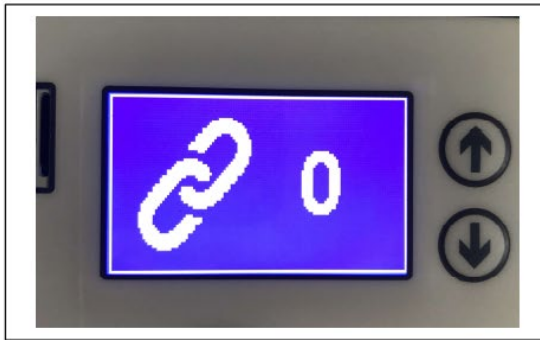
Channel 0: Factory reset
